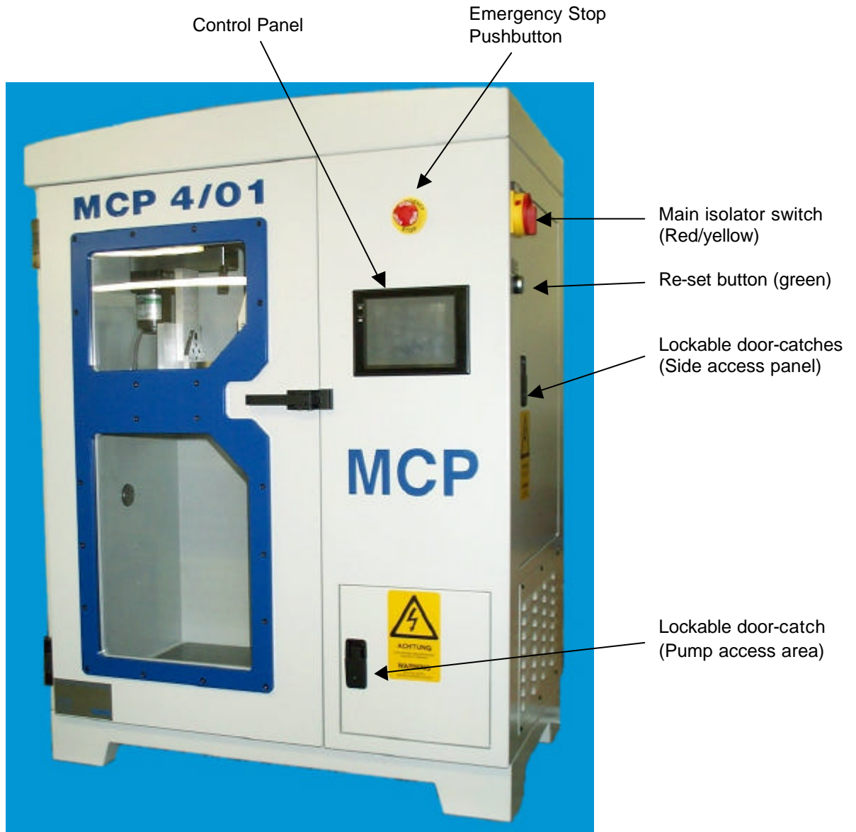
Fig. 1 General front view
