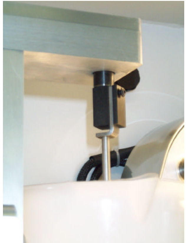
Fig. 5 Adjusting the paddle and holder
