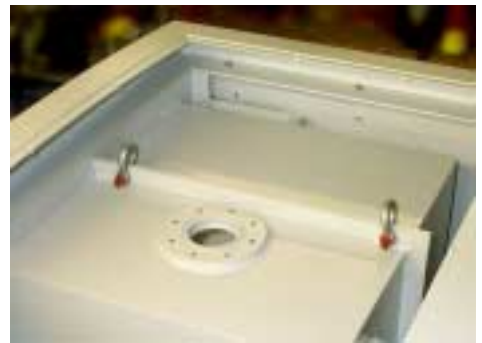
Fig. 4 Lifting Bolts in position.
