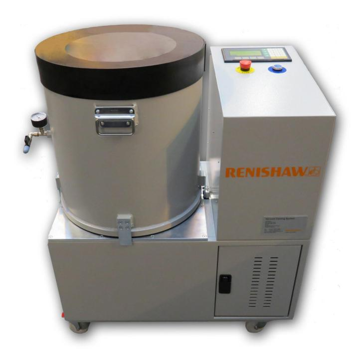
Thank you for purchasing a Renishaw Vacuum Mixer. The unit has been designed for use with the Renishaw series of silicone rubbers, high viscosity resins supplied for the manufacture of prototype tools via the Renishaw vacuum casting system.
