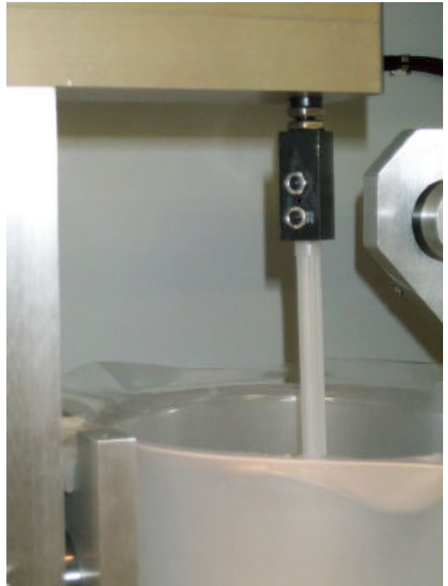
Fig. 5 Adjusting the paddle and holder
