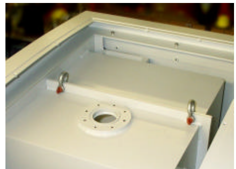
Fig. 4 Lifting Bolts in position.
